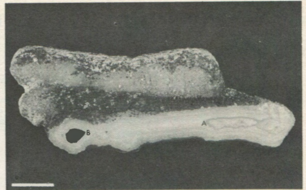
Fig. 4. A lengthwise slice of a silica stalactite, revealing carbonate growth lines (a) and a calcite crystalline aggregate (b). The speleothem surface is coated with euhedral quartz crystals 1 to 3 mm in diameter. Scale: 2 cm.
